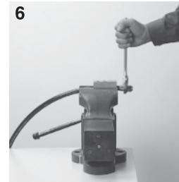
Insert the socket into the hose end and tighten it anti-clockwise with your hand. Then use the adjustable wrench to screw the socket to the position marked on the hose. Check that there is about a 2-3 mm space between the inner end of the socket and the hose end.
