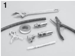
Prepare appropriate hose, coupling cutter, white pen, torque wrench, seal tape, and detachable jig.
