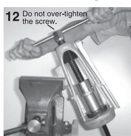
Attach the handle to the pressurization screw and rotate the handle clockwise to send the pusher down. Continue until the pusher touches the die.
