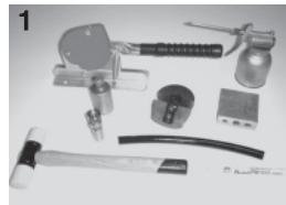
Prepare appropriate hose, swage coupling, pusher, die, hose cutter, holding die, lubricant\*, plastic hammer, scale, and white pen.
