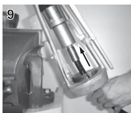
Insert the coupling, to which the hose is inserted, into the pusher.
