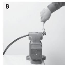
Tighten the nipple clockwise with your hand and use an appropriate adjustable wrench to slowly screw the nipple until its hexagonal part touches the socket.
