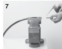
Remove the assembly from the vice and the holding die. Nip the socket with the vice and apply lubricant to the nipple thread and the inner surface of the hose.
