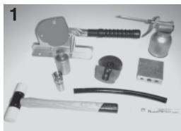
Prepare appropriate hose, swage connector, pusher, die, hose cutter, holding die, lubricant\*, plastic hammer, scale, and white pen.
