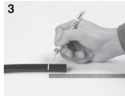
Measure the insertion length of the hose with a scale and mark the hose at the insertion length with the white pen.
