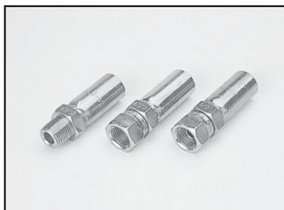
The swage coupling is attached to the hose by swaging. The coupling and the hose can be easily swaged (assembled) with a manual assembling tool [Mark10], or a hydraulic assembling machine [Mark9].
