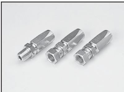
The reusable coupling is used to screw in a hose. On-site assembling is possible and the detached coupling is reusable.
