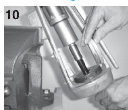
Put the other mate of the die on the base. Turn the die clamp to lock the die and fix it firmly.
