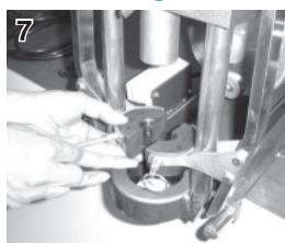
Attach the die onto the die fixing arm using the fixing pin.
