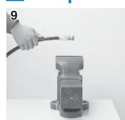
After finishing the tightening of the nipples, check for deformation of the core tube by inserting a checking stick into the coupling.
