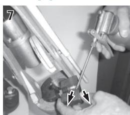
Apply lubricant to the inner surface of the die.
