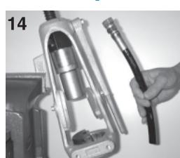
**Caution** Before putting the die in storage, remove dust from the inner surface and thinly grease it to prevent rust.
