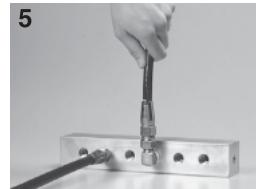
Insert the hose into the coupling until it meets the marked position. Repeat the same steps 2-5 for the other end of the Campucka.
