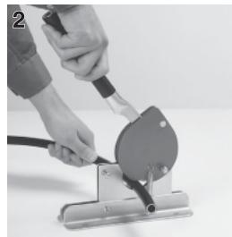
Determine the cutting length of the hose based on the hose assembling length and cut the hose squarely using the special hose cutter.
