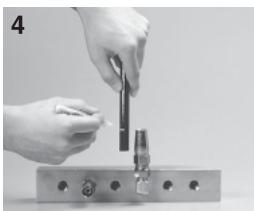
As shown in the figure, mark the hose with a white pen, fitting the hose edge to the groove mark of the socket.
