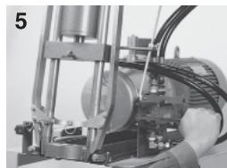
Push the operation lever to the back to lift up the pusher holder.
