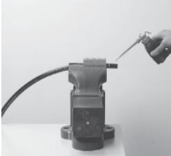
Nip the hose with the holding die, leaving the length of hose end to be inserted into the socket, and fix it in the vice. For easy screwing, apply lubricant to the surface of the hose end.
