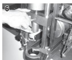
Attach the pusher to the pusher holder. Fix the pusher by turning the screw of the pusher holder so that the pusher can freely rotate.
