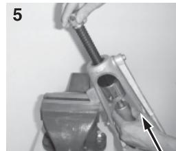
Fix the rib of Mark 10 on the vice and pull out the pressurization screw to the longest position. The die clamp should be open as shown in the figure.
