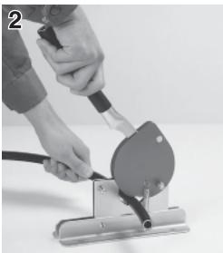
Determine the cutting length of the hose based on the hose assembling length and cut the hose squarely using the special hose cutter.
