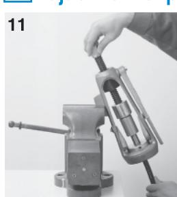
Hold the hose beneath the die base with your left hand. Pushing the coupling toward the pusher, turn the pressurization screw clockwise with your right hand to send the pusher down.
