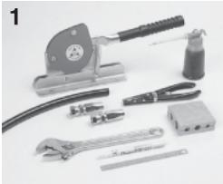
Prepare appropriate hose, coupling, hose cutter, holding die, lubricant\*, adjustable wrench, scale, and white pen.
