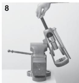
Fix a mate of the die onto the tapered base.
