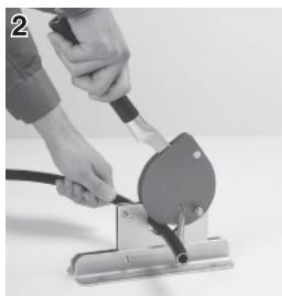
Determine the cutting length of the hose based on the hose assembling length and cut the hose squarely using the specific hose cutter
